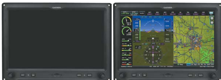
G3X Touch Full-Screen Reversionary Mode (Failed PFD)
